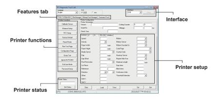
(3) The detail functions in the Printer Function Group are listed as below.
