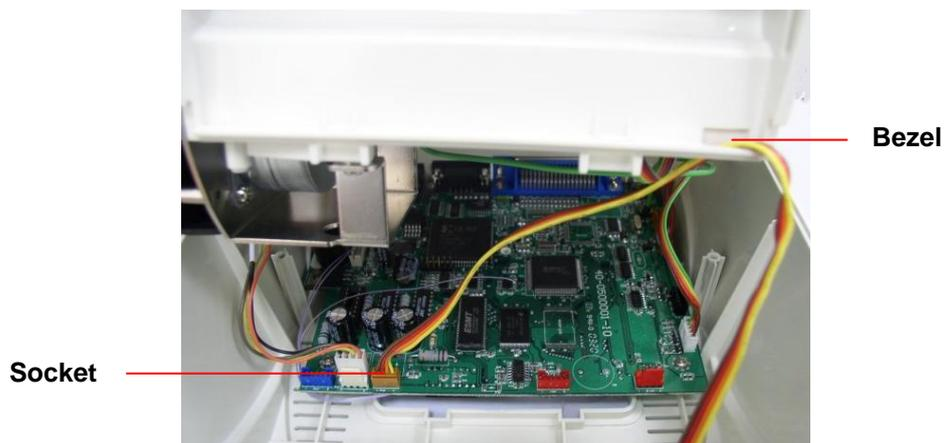
11. Reassemble lower inner cover back to the lower cover.
